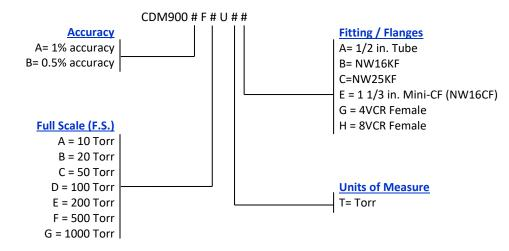
Example: CDM900BFAUTB (CDM900, 0.5% accuracy, 10 Torr F.S, Torr units of measure, NW16KF fitting)
