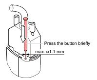
After zero adjustment the gauge automatically returns to normal measurement mode.
