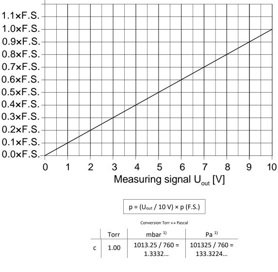
Example: Gauge with 10 Torr F.S. Measuring signal U<sub>out</sub> = 6 V
