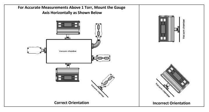
Mount the CVM201 with port down, if possible, to help minimize the effect of any particles or condensation from collecting in the gauge.
